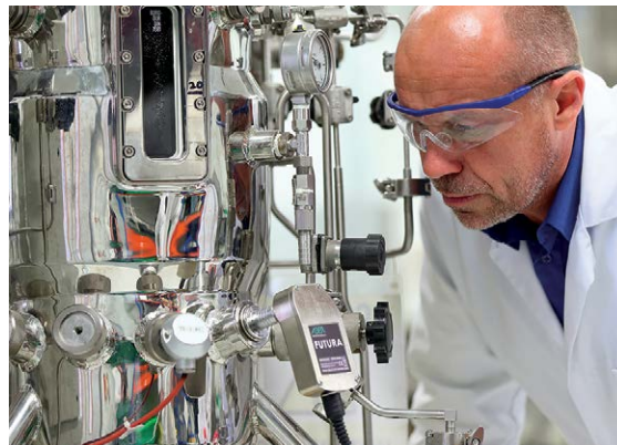
Figure 2: Aber electrodes creating an electrical field and measuring capacitance of live cells
