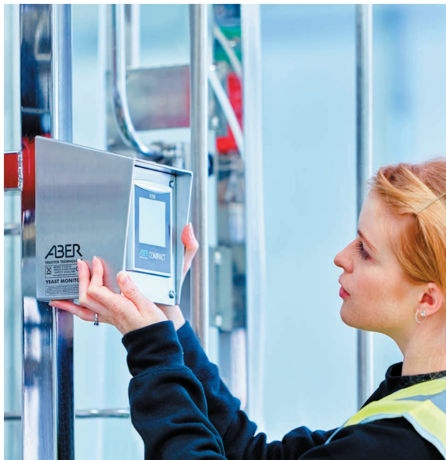
Aber's Compact v350 Touch Screen being installed at a brewery
